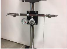
• Attach one end of oxygen hose to the back of machine. Attach other end of hose to regulator on yoke.
