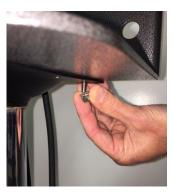
• Use a 5/32" Allen wrench and 7/16" wrench to securely tighten all bolts.
