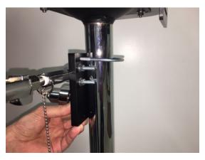
Place flat washer, star washer, and nut on U-bolt. Align yoke parallel with machine. Adjust height of bracket on
