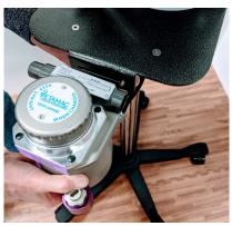
Connect inlet and outlet adapters to the vaporizer, routing the Norprene tubing under the machine.
