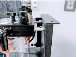
• Secure to the chassis by inserting the three-arm bolt into the hole in the back of chassis and tighten.
